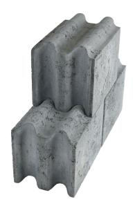
Size: 150 x 200 x 150 mm Weight: 17.5 kg Pallet: 72 pcs, 1280 kg Consumption: 33.3 pcs/m² Dry density: 3800 kg/m³
